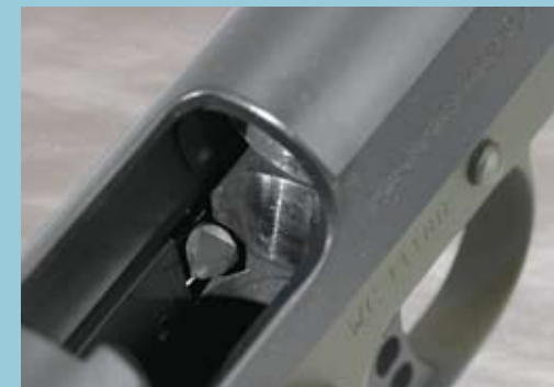
A hollow plunger (above, l.) retains the Wilson's recoil spring and one-piece guide rod. The pistol's polished feed ramp on its steel frame (above, r.) ensures flawless feeding of a variety of bullet types. We experienced no malfunctions of any kind.
