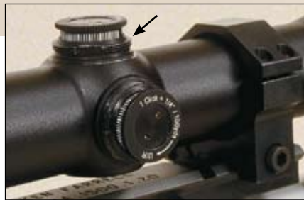
The windage and elevation turrets feature a movable sleeve (arrow, above) with markings that can be zeroed against a reference mark on the scope body. An easily focusable eyepiece (r.) is a boon for those needing diopter changes.
